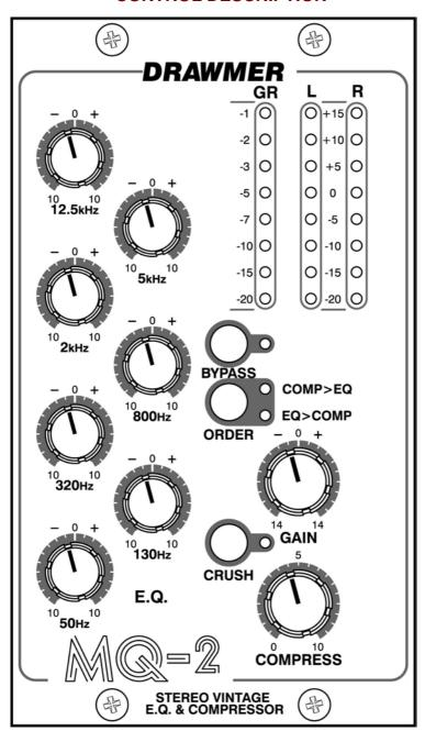
As the MQ-2 is stereo all controls effect the left and right settings simultaneously.
