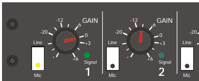
**GAIN** Volume preset for both the microphone and the stereo-line input.
