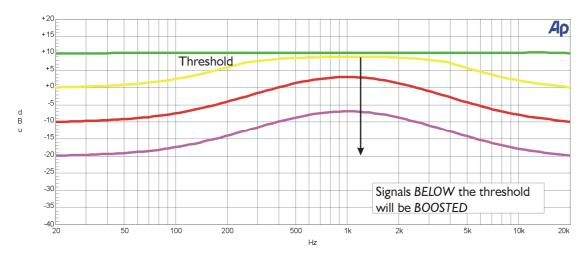
Signals above the threshold pass unaltered but, as the signal drops below the threshold, frequencies around the 1kHz region will be progressively boosted (or expanded). How much boost is applied will depend on the ratio set and how far below the threshold the signal actually is.
