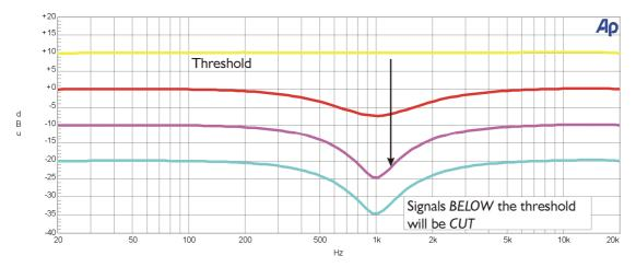
Signals above the threshold will pass flat, but as the level decreases, those frequencies centred around IkHz will be cut or expanded. The amount of gain reduction applied depends on how much the signal drops the threshold and the ratio set – a 2:1 ratio would mean that for every drop of IdB below the threshold, the band centred around IkHz would drop by 2dB.
