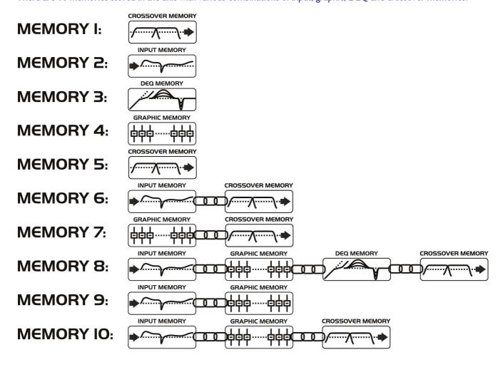
As can be seen, different memory locations contain different combinations of the three memory types available. If it is required to recall a location that contains everything (Input, Graphic, DEQ, and Crossover settings), this will limit the selection as shown overleaf...
