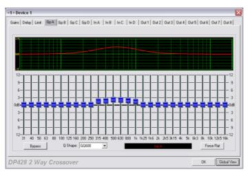
Consider the group of faders gently boosted as shown below, with the "GQ600" behaviour selected. As can be seen, the filters' responses have combined to give a smooth lift in response across the entire region. The overall level is considerably higher than the individual amount of boost applied to any single band.
