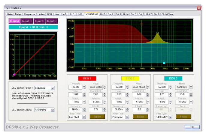
The AudioCore screenshot above shows a DEQ screen with band I set to operate as a low shelving filter in "Boost Below" mode – this will progressively introduce the low shelving response to the incoming audio as it drops below the set threshold. Using this and another band set to a high self will allow a classic loudness curve to be realised, but with the added advantage of being related to the audio signal, not just determined by the gain control of the channel.
