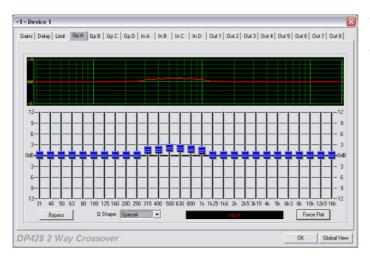
The same bands have been boosted in the example below this, but the behaviour has been set to "Special". The ripple in between bands is now obvious, due to the bandwidth not having widened at low level boosts. However, the overall level is much closer to the highest maximum filter's boost.
