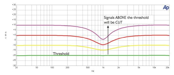
Signals below the threshold will pass unaltered, but as increasing signal is applied, those frequencies centred around 1kHz will be cut or compressed. The ratio in the above example is set at 2:1 so, as with any compressor, the amount of gain reduction applied depends on how much the signal exceeds the threshold. The red line represents a signal at 0dB, which is 20dB above the threshold. At 1kHz, therefore, the signal has been compressed to –10dB or 2:1.
