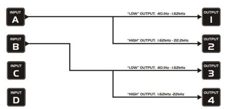
4 x 1 way crossover: Each input is routed to a corresponding output A to 1, B to 2 etc. Crossovers filters are bypassed.
