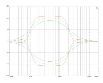
To create a flat-topped EQ filter response such as that shown to the left, use two EQ bands, BOTH configured as low shelves. For an overall BOOST, set the Lower frequency filter to BOOST the desired amount, and the Upper frequency filter to CUT by the same amount.
