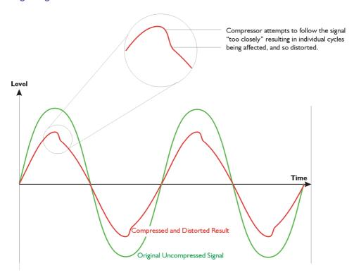
The compressor and DEQ release time has been deliberately restricted to a minimum of 45mS to prevent excessive distortion on low frequency signals, even with fast attack times and high ratios. None the less, it is still possible to introduce some distortion if care is not taken with the settings. The best way to ensure that the signal is not being excessively distorted is to make good use of the 'BYPASS' button, constantly comparing the original signal with the effected version.
