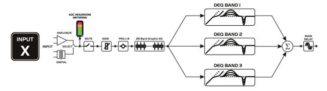
The outputs of the bands are then summed again before being passed on to the main (base) delay module. The bands do not interact with each other and so overlapping frequency bands cannot cause unexpected overall effects.
