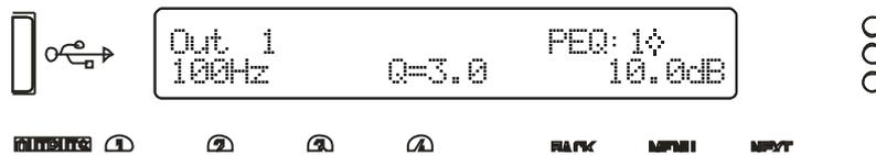
Parametric bands missing? If bands 6 and 7, or 8 and 9 are missing when editing, it is because they are being utilised by high order crossover filters – high pass filter orders above 24dB/Octave will disable and hide bands 6 and 7, and low pass filter orders above 24dB/Octave will similarly remove bands 8 and 9.
