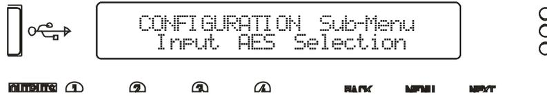
Use the encoder or BACK and NEXT keys to find the Input AES Selection option and press ENTER.
