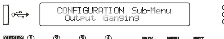
Use the encoder or BACK and NEXT keys to find the Output Ganging option and press ENTER.
