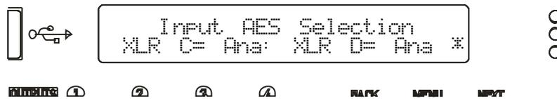
Use the encoder or BACK and NEXT keys to cycle between the four combinations, of analogue (Ana) or Digital (AES). Press ENTER to confirm the choice, and again to confirm if changes have been made.
