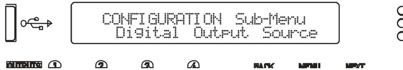
Use the encoder or BACK and NEXT keys to find the Digital Output Source option and press ENTER.
