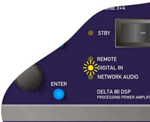
If the AES input(s) have valid stable signals and there are no other issues, the LED will not be flashing.
