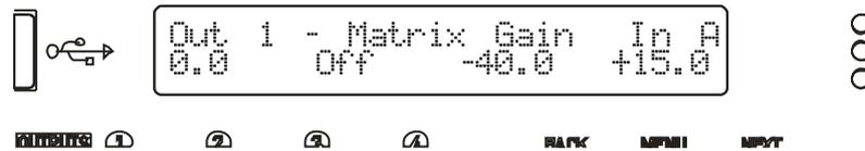
Initially, the “send” level from Input A will be selected – press ENTER to jump to the next “send” level for this output. Range is from -40dB to +15.0dB, with Mute one step below -40.0dB, whereupon the display will show “Off” as for Input B’s send level in the above example.
