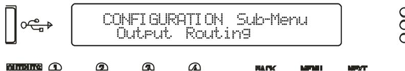
Use the encoder or BACK and NEXT keys to find the Output Routing option and press ENTER.
