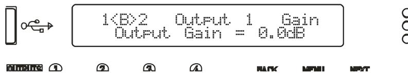
In this example, the bridged pair are outputs 1 & 2 and this will be displayed if EDIT is pressed on either output channel.
