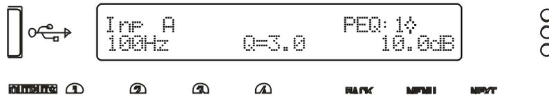
A filter must be in Bypass before its type can be changed. Once bypassed, the ENTER key will allow access to the type list and this can be adjusted with the encoder, scrolling through the types listed above.
