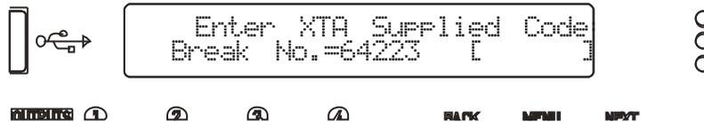
Make a note of the “Break Number” shown (64223 in this example) and contact us with this – we can then supply the code to unlock your amplifier.
