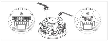
Connect the wiring by attaching the cables to the terminal block connectors and plugging them in to the CELO8S. Make sure the connectors are secured by tightening the set screws.
