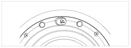
Depending on the acoustical properties of your room and placement of the subwoofer, the sub can be better integrated in your room when switched to either  $0^{\circ}$  or  $180^{\circ}$ . We recommend  $0^{\circ}$  when all speakers are mounted in a flat wall or ceiling.
