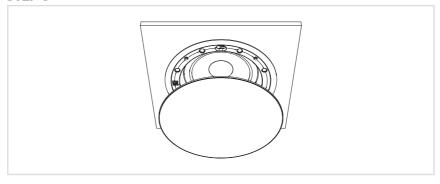
Attach the grill. Thanks to the magnets, it will snap in place.
