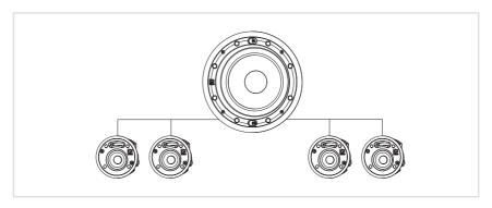
The CELO8S features an integrated stereo crossover, enabling you to connect your satellites. Two or four 8 ohm satellites can be used as well as eight 16 Ohm satellites.
