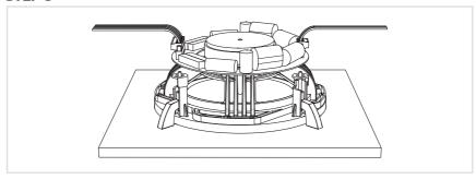
Tighten the screws for proper fixation of the speaker.
