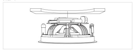
Make sure the mounting clamps are fully bended inwards, allowing the speaker to fit through the cut out. Insert the speaker into the cut out and tighten the mounting screws. A quarter turn is enough to flip out the mounting clamps, locking the speaker in place.
