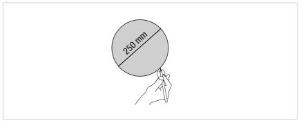
Cut a hole on the mounting location in the ceiling. Make sure the diameter is matching the cut—out measurement for the installing loudspeaker.
