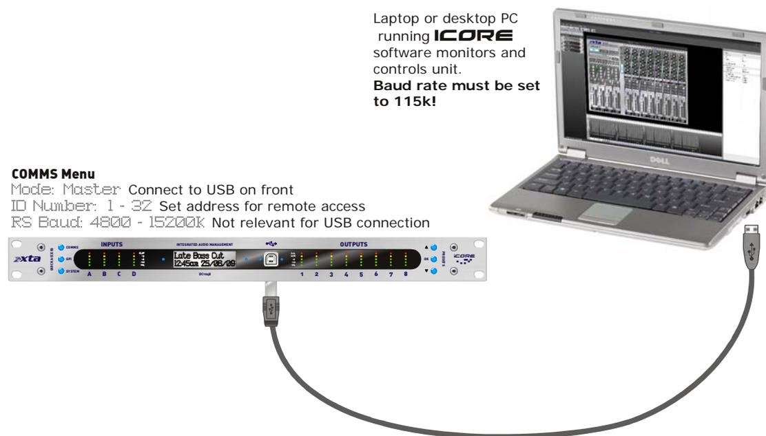
Set the options in the unit's COMMS menu according to the diagram, that is
