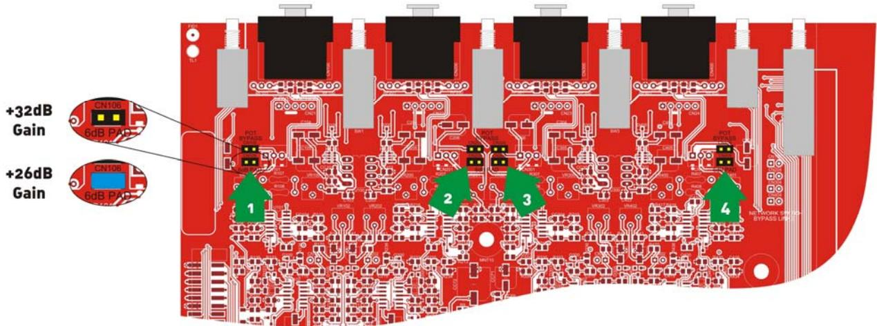
Remember, setting higher gain does not change the maximum available power but changes the level of signal input to achieve maximum power. In any case, provided that the input signal is less than 20dBu/7.7V, the built in limiter circuit will prevent distortion within the amplifier.
