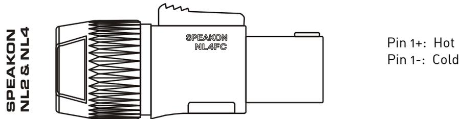
Additionally, Channel 1 Speakon connector carries Channel B2 output on Pins +2 & -2 to allow easy bi-amping or bridged operation using a single NL4 connector. Similarly, Channel 3's Speakon connector also carries Channel 4 output.
