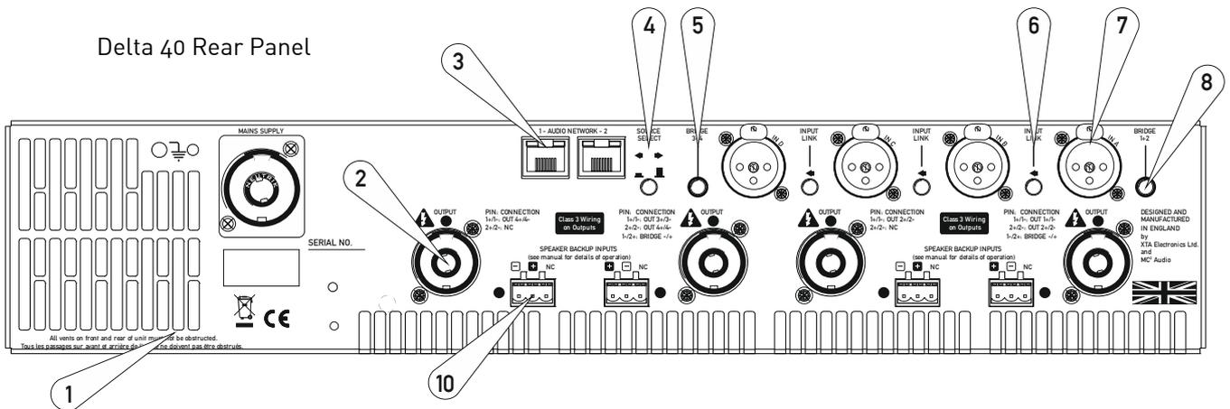
1: Fan outlet: The variable speed fans suck air in through the front vents and out through the back of the amplifier. Please see maintenance on page 19 for recommendations on how to clean this and the front foam sections.
