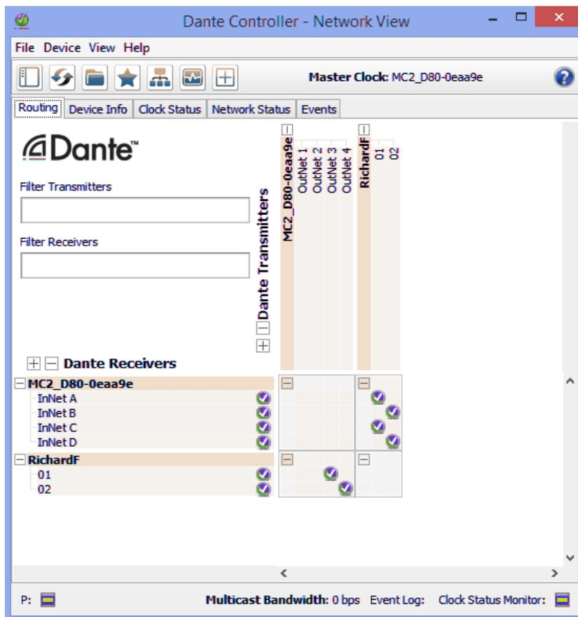
Note that the rear panel “Link” switches do not function in Network Audio mode as any linkage can be set up as part of the source selection within Dante Controller. Front panel “Link” LEDs will also extinguish.
