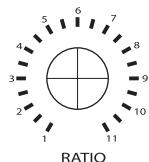
● **RATIO** - Controls the Compression Ratio from very gentle, around 1.5:1 to a very good squash around 10:1. This control as with many of the GERM Comp parameters were set/designed by extensive listening. We did not “do the math!” Instead we adjusted the individual settings while listening to various pre-recorded tracks and used what sounded best on most sources.
