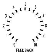
● **FEEDBACK** - The Feedback control is essential to the sound and function of this Comp. Audio amplifiers incorporate some amount of negative feedback which is where the output signal of the amplifier is fed back to its input. This affects the sound and function of the amplifier in many ways. THD, frequency response, gain and amplifier stabilization change considerably with varying feedback.
