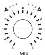
● WET/DRY MIX - The most surprising and effective feature of the GERM Comp, this lets you simulate parallel compression or sub-mixing in the unit. Mix the tight compressed sound together with the unprocessed original signal and get the best of both. Use this on any source to keep the compression from removing too much attack, transient, or intensity. Leave the attack and punch on your drums while adding in as much of the tight compressed sound as you need.
