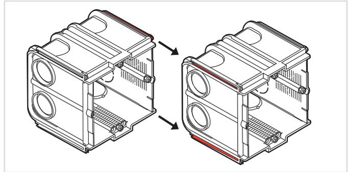
To use the WB45SI/FS with the NWP222, connect two flush mount boxes by sliding the rail connections on the sides to form the combined flush mount box.
