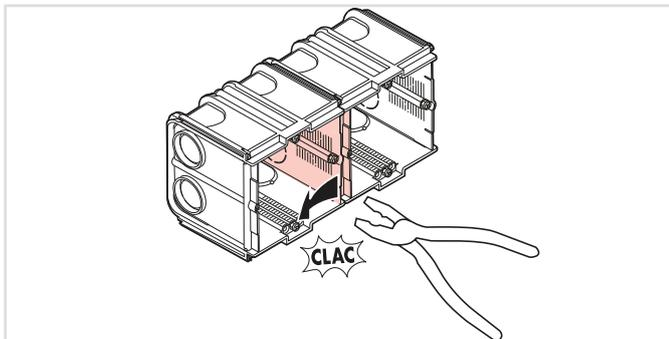
Remove the side walls between the combined flush mount boxes using a plier. This would open enough space for NWP222 to fit in.
