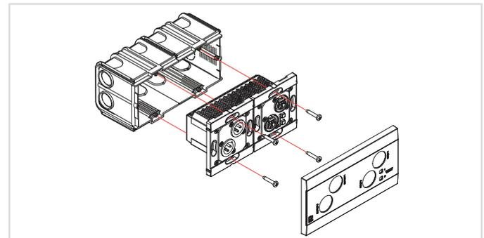
First, plug the twisted pair cable (CAT5E or better) into the wall panel. RJ45 port is located on the back of the wall panel. Then, install the wall panel into the single or combined flush mount box by tightening the screws of the wall panel using a screwdriver. Finally, snap and mount the front panel.
