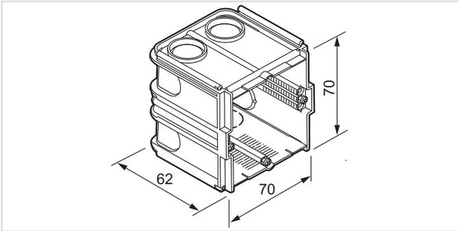
Prepare a hole on the mounting location in the surface. WB45SI/FS is compatible with the WP2xx series, NWPxxx series and NCP105. For the perfect fit with the NWP222, two WB45SI/FS shall be connected to each other.
