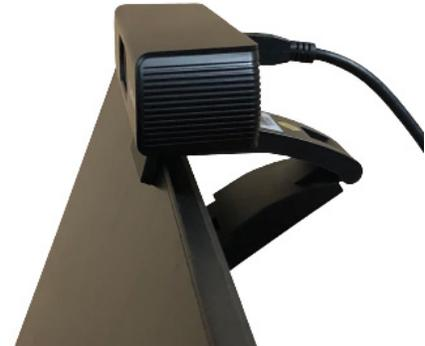
2. Connect the USB cable to the USB 3.0 Type B connector on the camera and the other end to a USB 3.0 Type A port on your computer. If your computer only supports USB-C ports, you will need a USB-A to USB-C adapter (not included).
