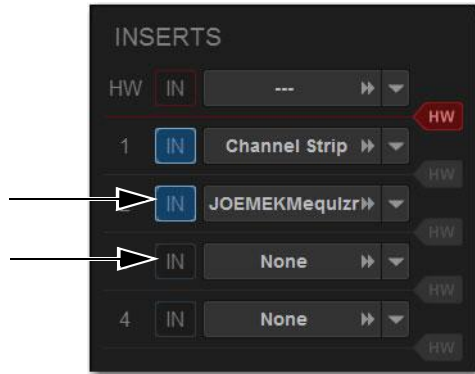
An engaged plug-in (top) and a disengaged plug-in (bottom)
