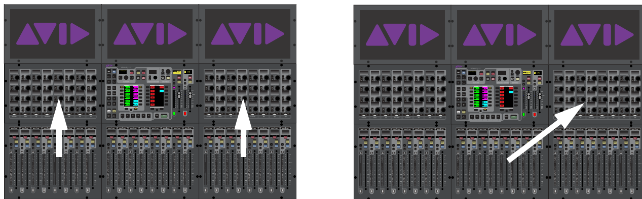
Selecting a channel below a CKM (left) and below the MLM (right) on an S6L-24D
