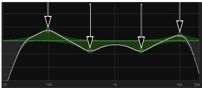
Drag the handles in the EQ graph display to adjust EQ
