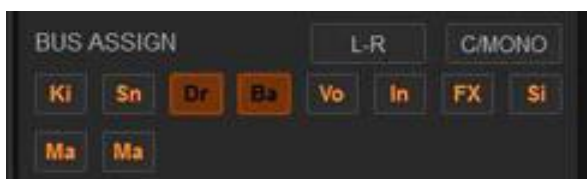
Bus Assign section showing a channel assigned to Groups 3 and 4 ("Dr" and "Bs")
