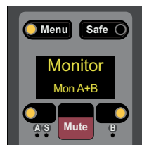
A channel display showing a channel routed to Monitor Bus A (Left) Bus B (center) and Buses A and B (right)
