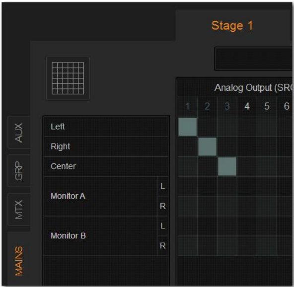
Mains patched to a Stage 64 hardware output
