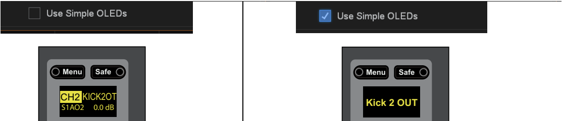
Channel display with Use Simple OLEDs disabled (at left) and enabled (at right)
