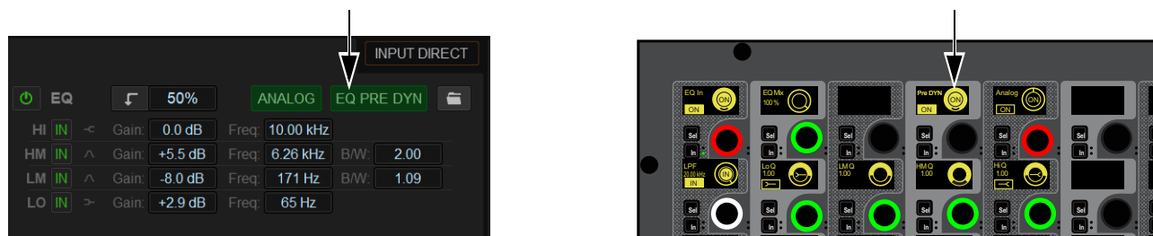
Inputs screen showing EQ PRE DYN button enabled/active (shown at left) and on a CKM in EQ mode (shown at right)
