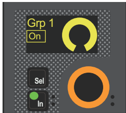
Encoder and display showing a channel assigned to Group 1 (left) and on-screen for the selected/attentioned channel (right)
