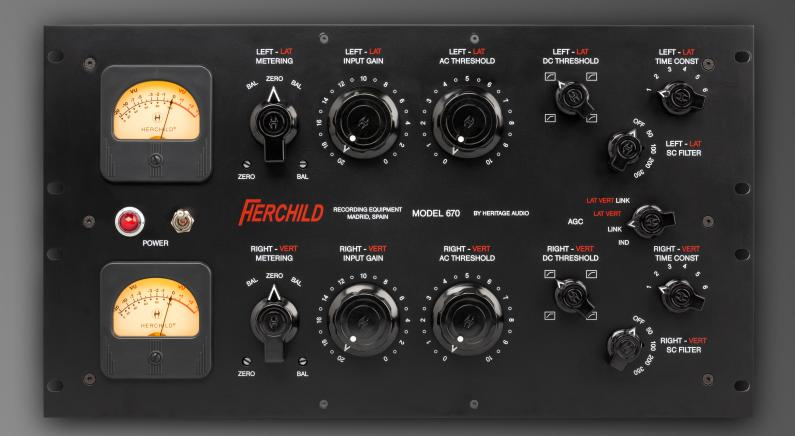
This is the two channel version that also offers the possibility to work in other modes of operation such as LINKED Stereo as well as MID/SIDE and MID/SIDE LINKED.
