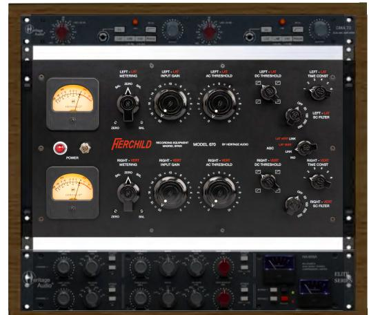
**Using the outer set of holes allows you to have 1/2 rack unit of space above and below.**
