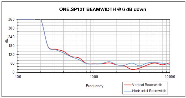
NOTE: These measurements were created using EASE software, which limits the bandwidth to 100 - 10,000 Hz that is critical for full-range loudspeakers
