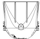
**Notice**: The enclosure must be installed with the logo positioned at bottom with a minimum downtilt of 5-degrees
