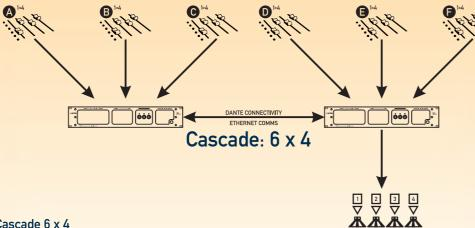
6 Sets, each with 4 inputs with full redundancy, and 4 outputs. Mic and stereo line inputs are available across all outputs. Console select and failover source selection remain independent on each unit. Output bus sums across both units via Dante.
