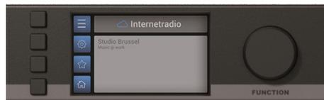
The functionality of the four tactile push buttons on the left side depends on the current mode and position in the menu structure. Icons on the left side of the display are indicating the current functionality linked with the buttons.
